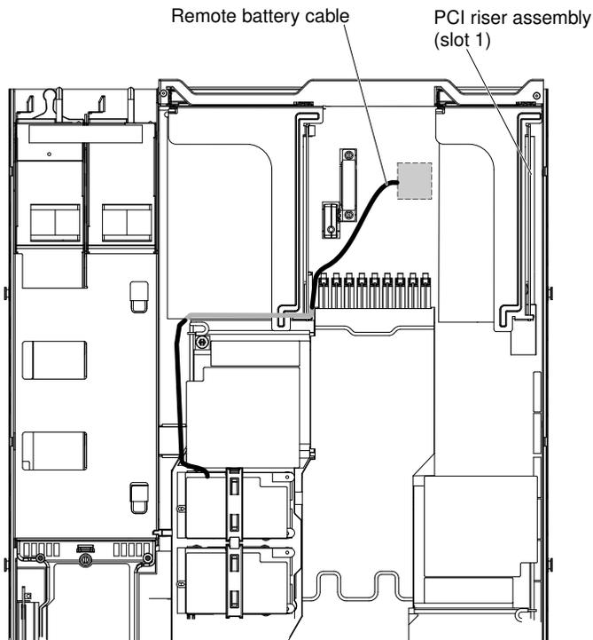
Figure 68. Cable connection
