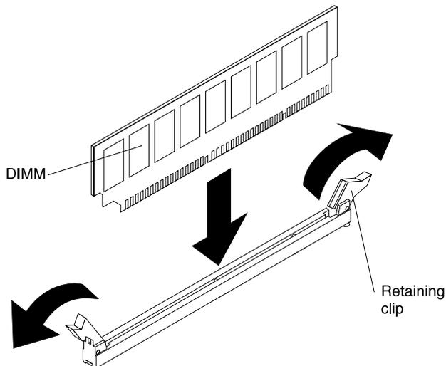
Figure 32. DIMM installation
