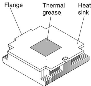
Figure 83. Thermal grease
