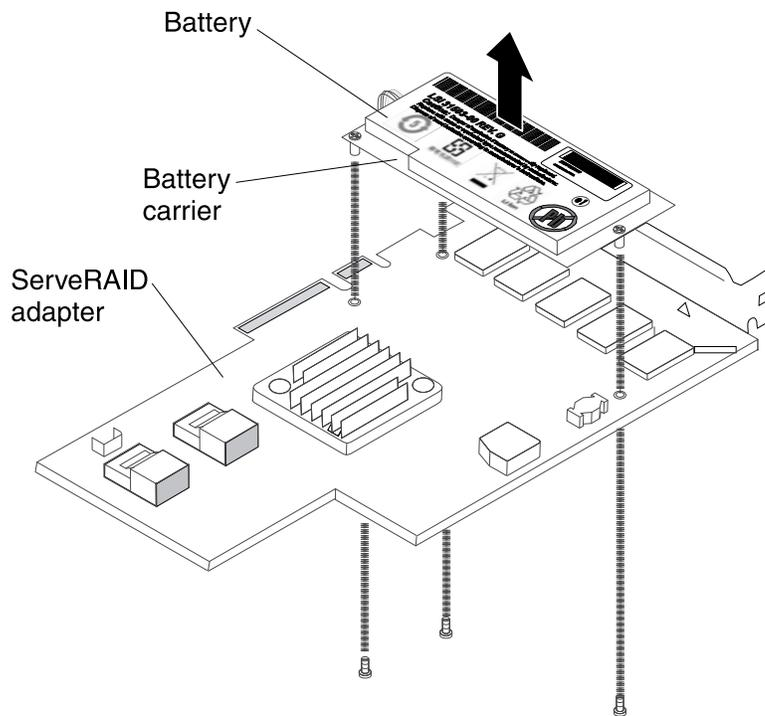
Figure 64. Battery removal
