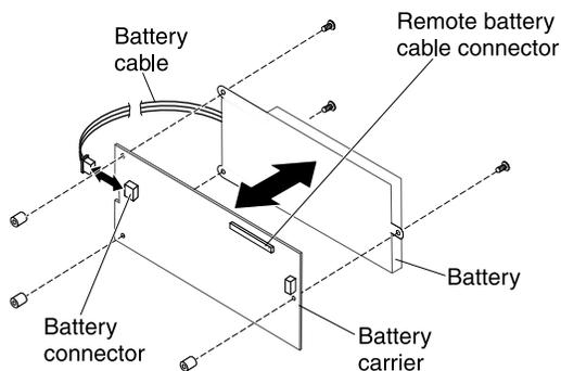
Figure 69. Cable connection
