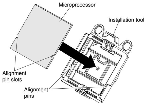
Figure 79. Microprocessor alignment
