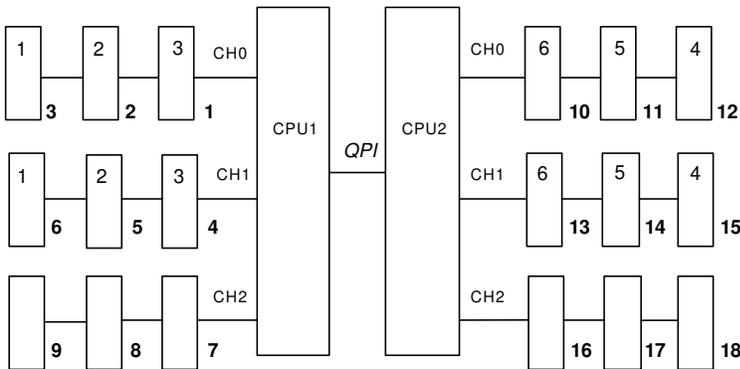
Figure 30. Memory channel interface layout
