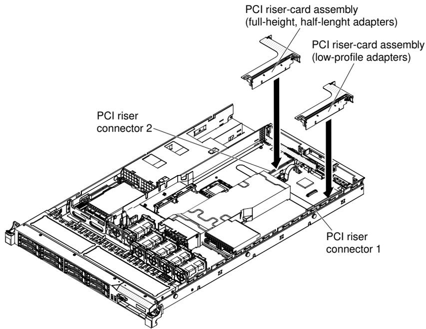
Figure 41. PCI riser-card assembly installation
