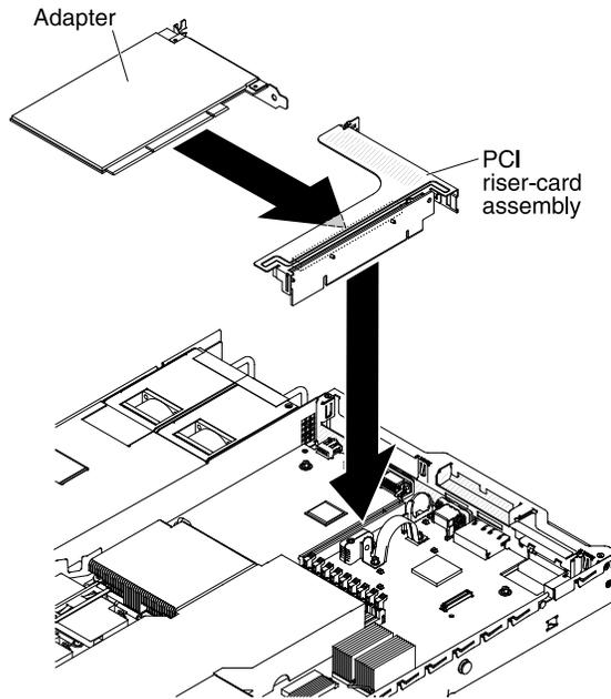
Figure 42. Adapter installation
