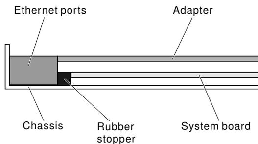
Figure 62. Adapter installation
