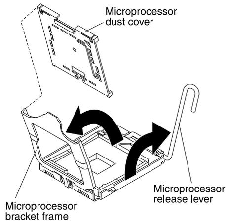
Figure 78. Dust cover removal
