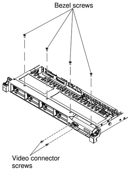
Figure 75. Screws removal
