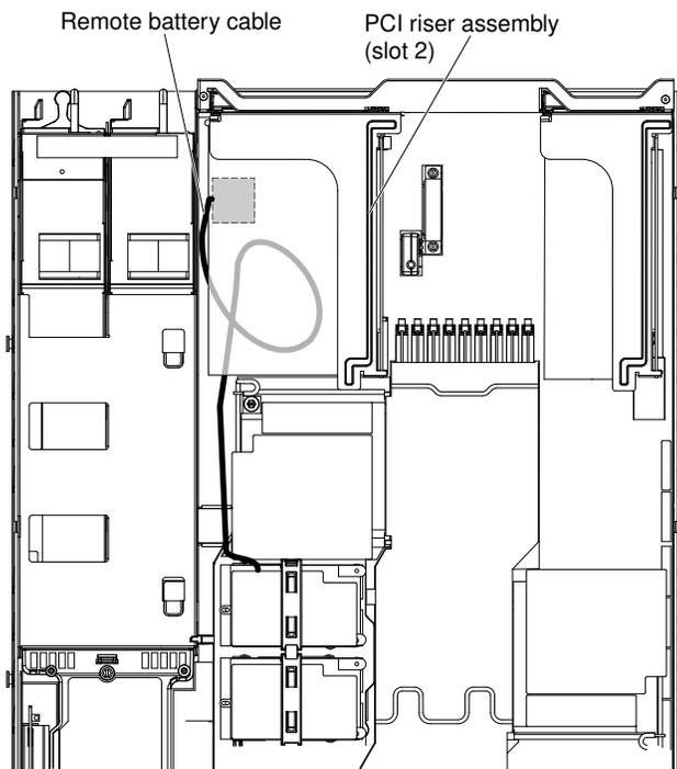
Figure 67. Cable connection
