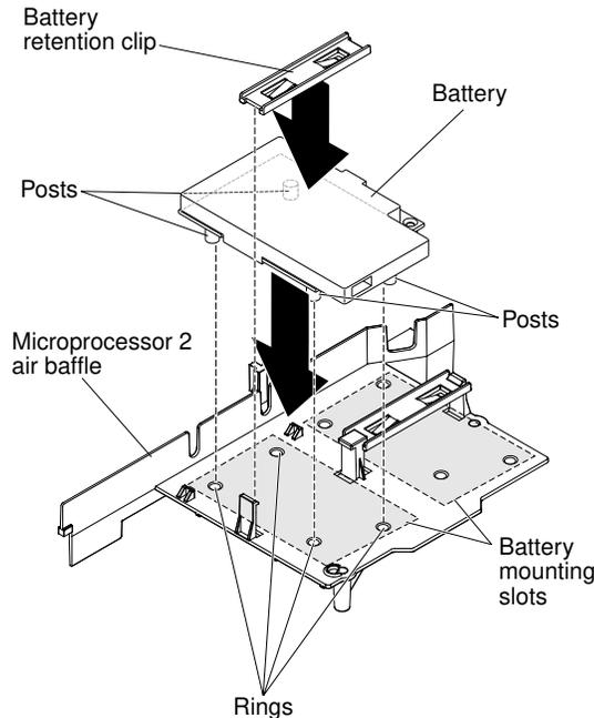
Figure 70. Battery installation
