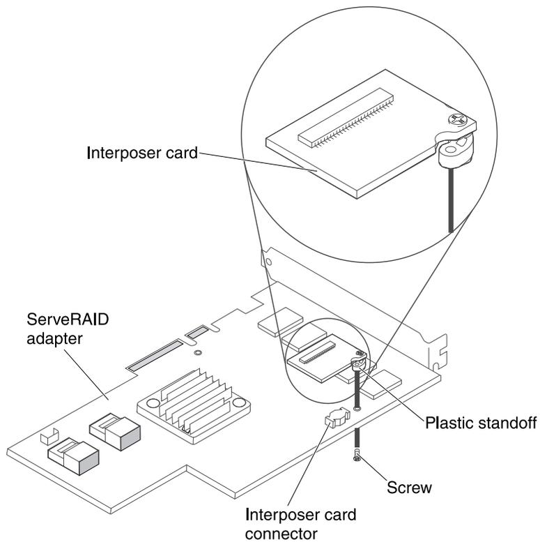
Figure 65. Interposer card installation
