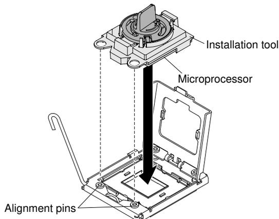
Figure 81. Microprocessor installation
