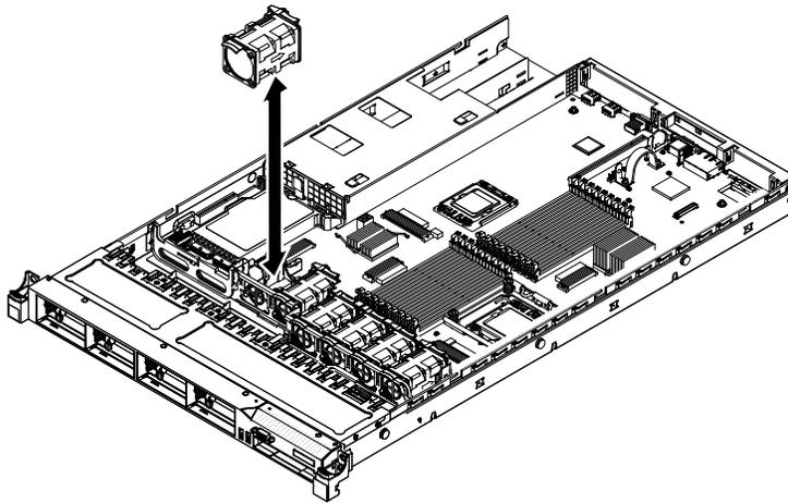
Figure 53. Fan installation
