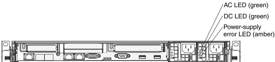
Figure 12. AC power-supply LEDs
