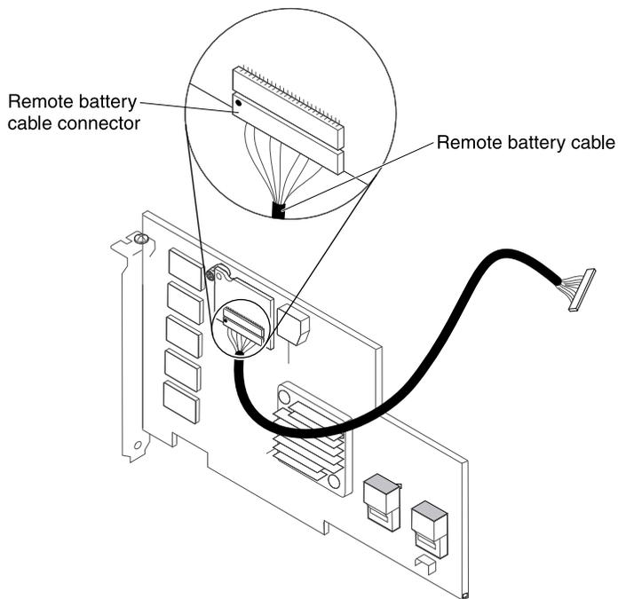
Figure 66. Cable connection
