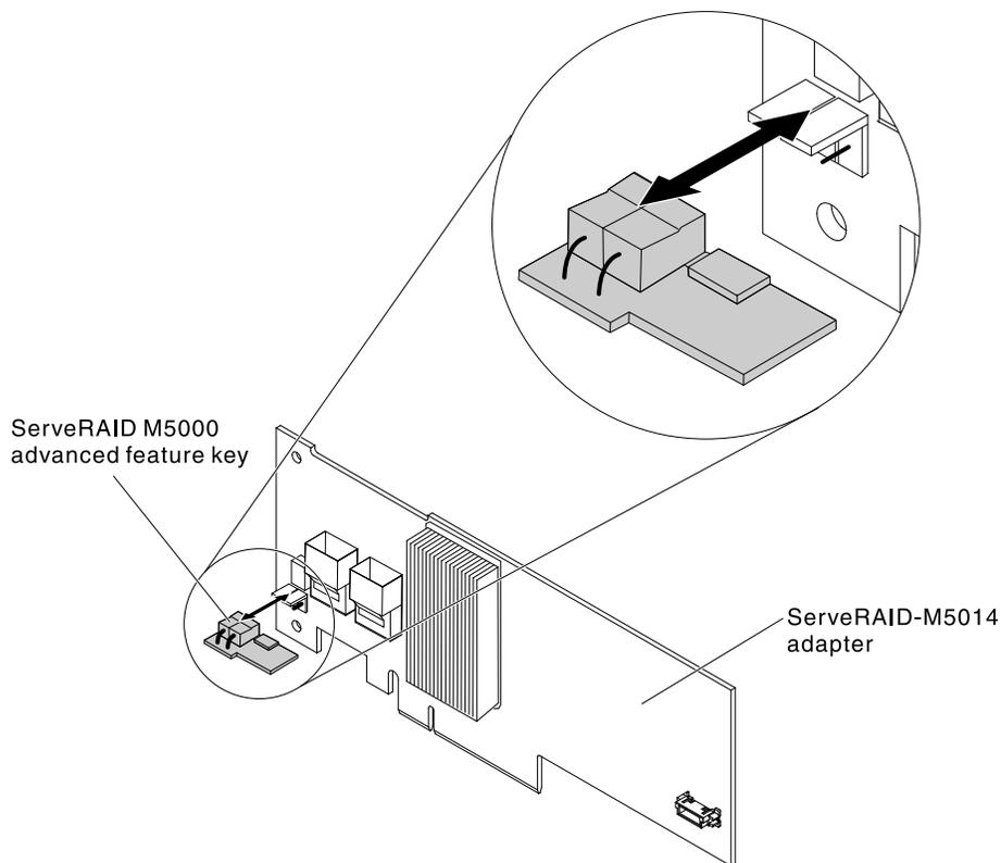
Figure 51. ServeRAID M5000 advanced feature key installation
