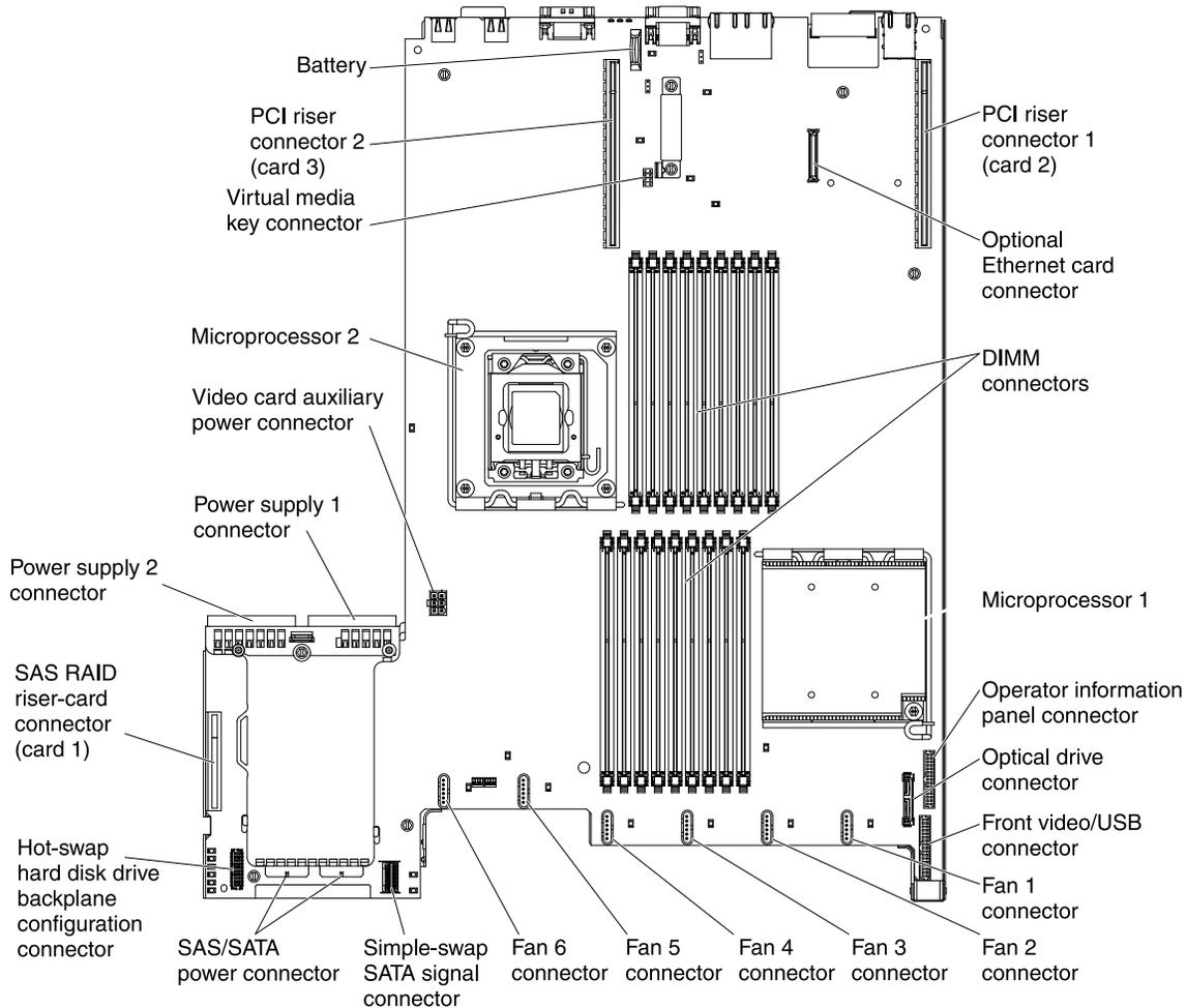
Figure 15. System-board internal connectors
