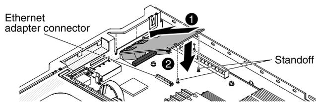
Figure 61. Adapter installation
