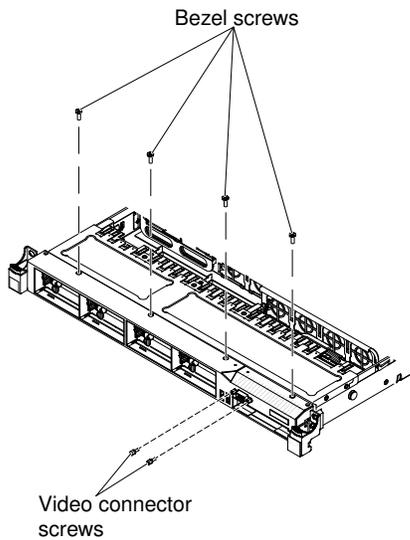
Figure 71. Screws removal
