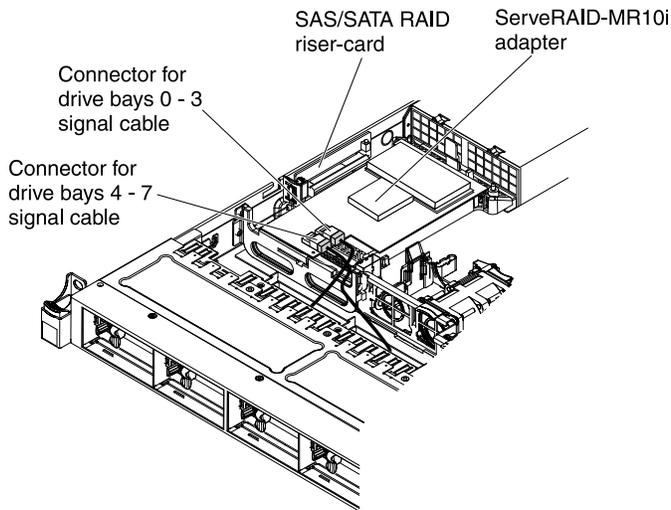
Figure 20. ServeRAID adapter cable connection
