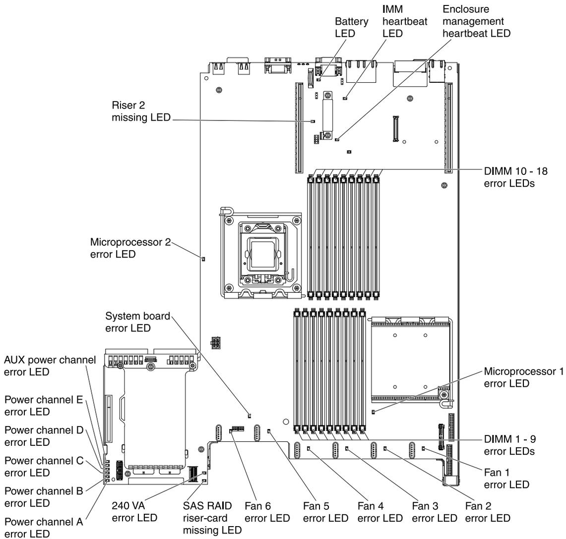
Figure 18. System-board LEDs
