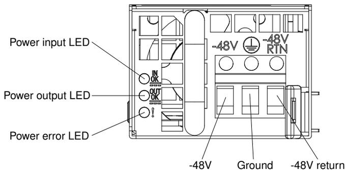
Figure 13. DC power-supply LEDs
