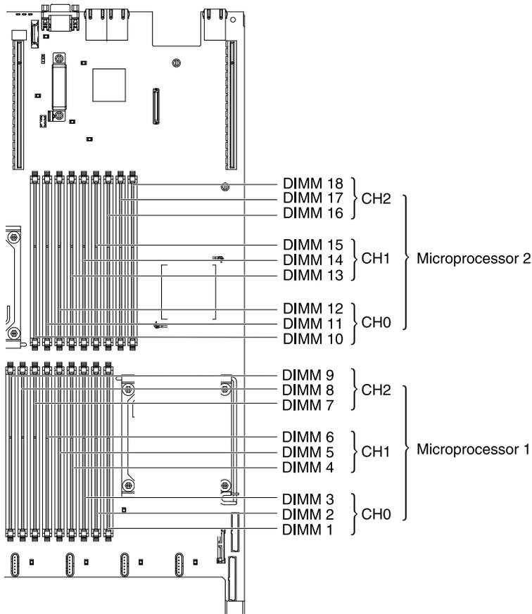
Figure 29. DIMM connectors location
