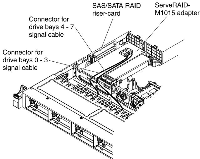
Figure 48. ServeRAID-M1015 adapter cable connection
