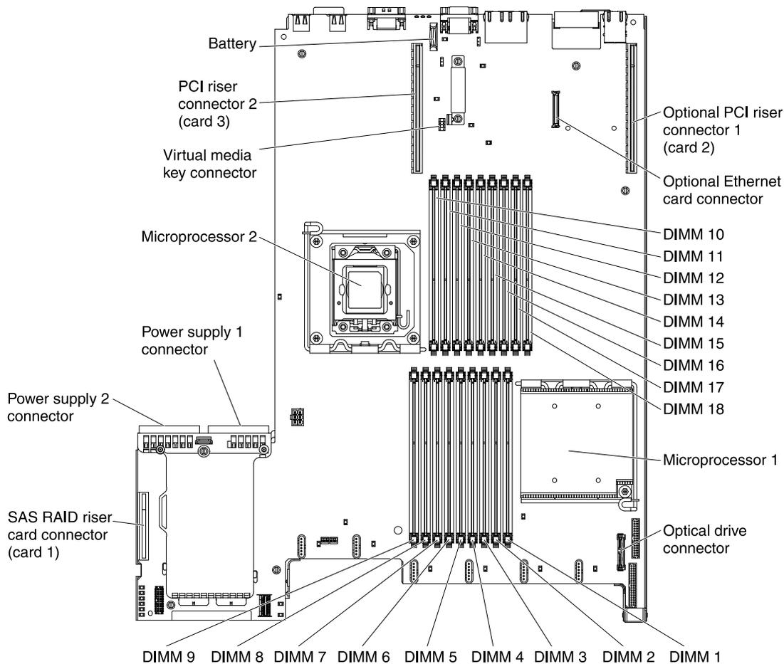
Figure 19. System-board optional device connectors
